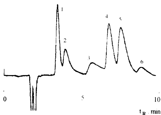
Fig. 3. Separation of a mixture of alkali and alkaline earth metal ions. Column, Lys-SiO 2 (150 mm × 4 mm I.D.); injection volume, 20 μl; eluent, 5 mM HNO 3 ; flow-rate, 1.5 ml/min. 1 = Li + ; 2 = Na + ; 3 = K + ; 4 = Ca 2+ ; 5 = Sr 2+ ; 6 = Ba 2+ .
